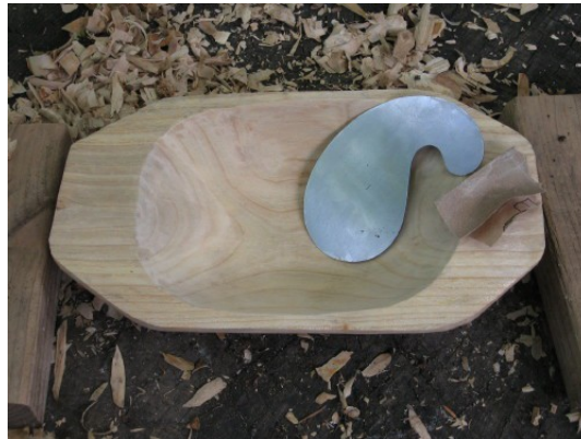
Oliver's tool doubles for the gooseneck scraper used by fine woodworkers. Image: http://outdoors.magazine.free.fr/spip.php?page=print_article&id_article=333
