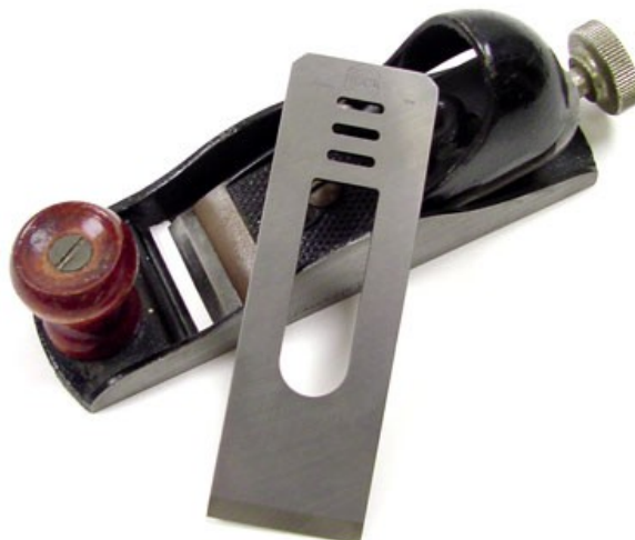
Typical plane bit, showing long opening.
