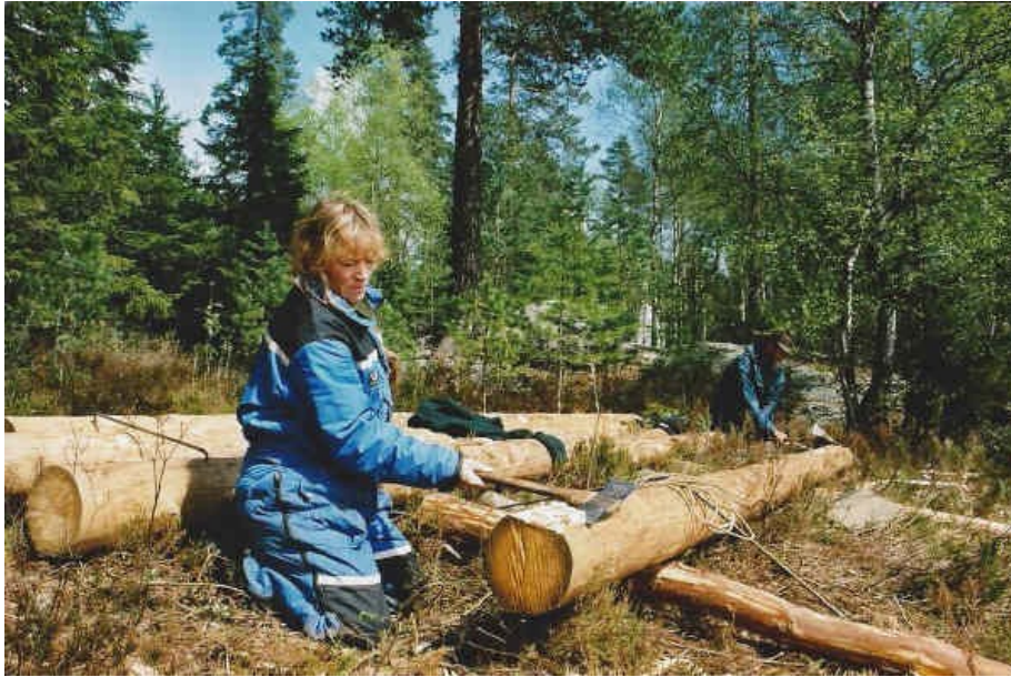
Heidi Dammann and Oliver begin working on the raft. Note the steel dog holding the logs behind Heidi. The raft will be pushed down the skids into the water later. Photo: Anne Kirsti Augestad.
