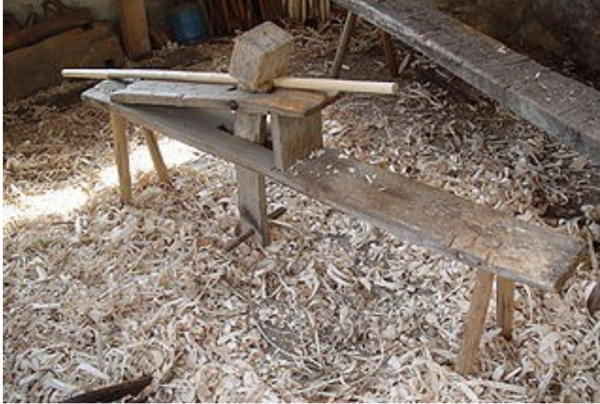
Shaving horse, as used by some artisans in Cantabria (Spain). The user pushes the pedals forward to clamp the work in place. Image source: http://en.wikipedia.org/wiki/Shaving_horse
