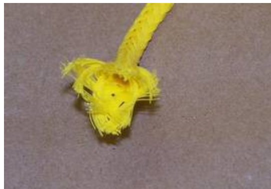
Hollow braided rope has no core.
