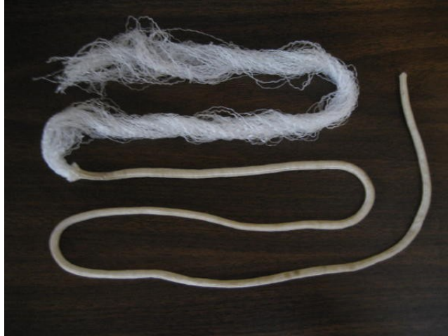
Parachute cord with the inner threads partially extracted. The threads on this particular piece of cord were too fine to be useful for sewing. Image: Ole Wik
