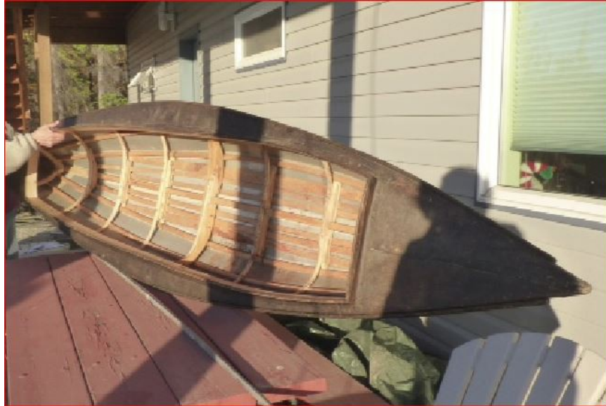
This image of Oliver's larger kaynoe shows the covered deck and the cockpit. This model does have a coaming. Image: Dorene Cameron Schiro
