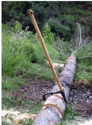
Homemade log peavey, used for rolling logs. Image: http://lumberjocks.com/projects/8271
