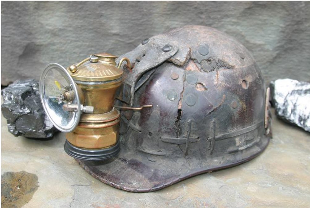
Miner's helmet with attached carbide lamp. Image: http://www.ironminers.com/mineforum/viewtopic.php?t=730
