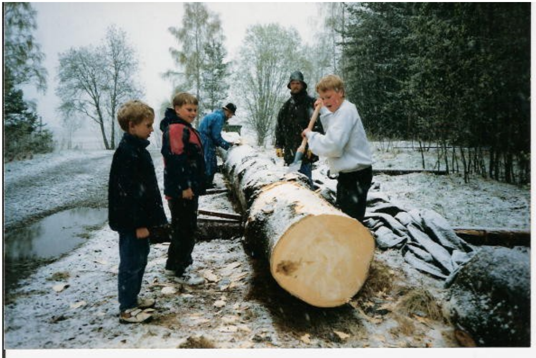
Beginning work on the dugout canoe. Oliver is at the far end, in blue. Rein Damman is wearing the rain suit. Dyre Dammann is wielding the slick to remove bark. Two young friends look on. Image: Heidi Dammann
