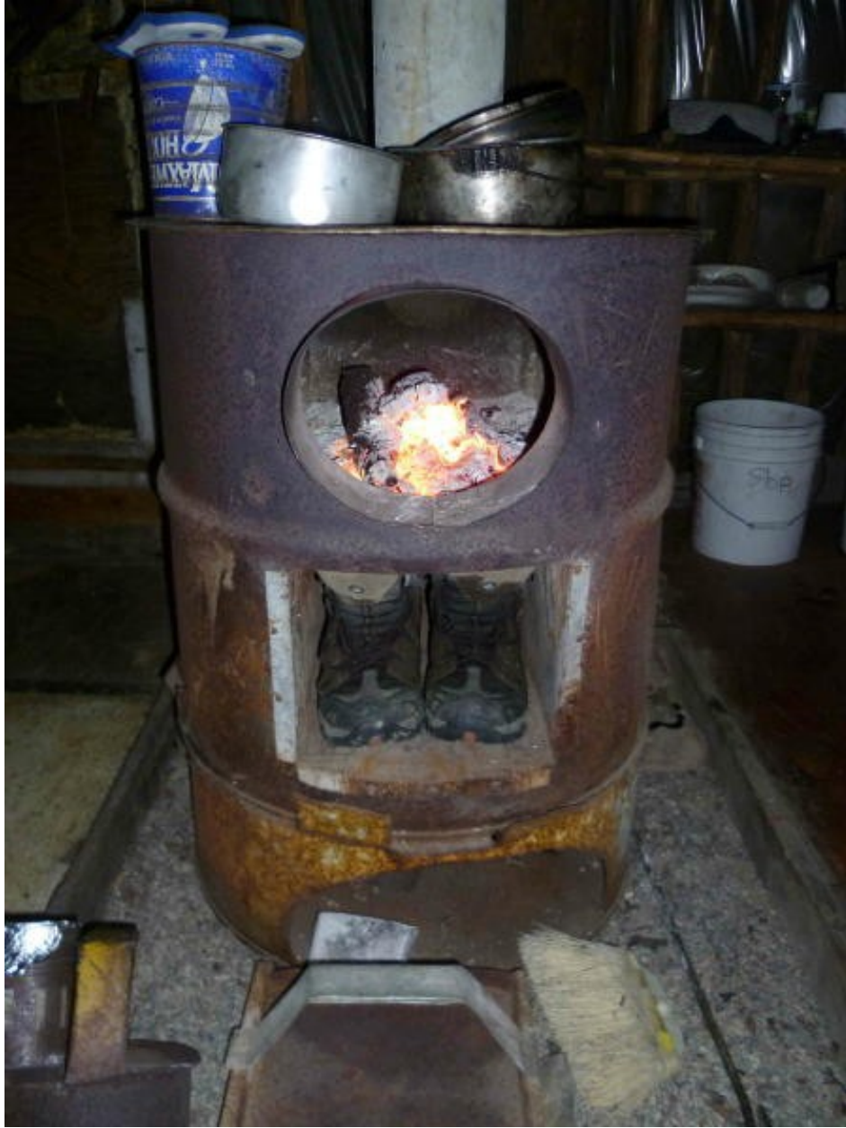
Oil barrel stove with boots drying in the oven. The heat from the firebox circulates down under the oven and back up the other side before reaching the stovepipe.
