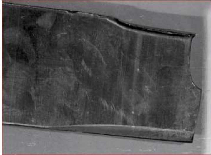
Another example of an improvised side-cutting chisel. Note the pounded edge on top, cutting edge on the bottom. This is a handy tool for cutting the top out of an oil drum.
