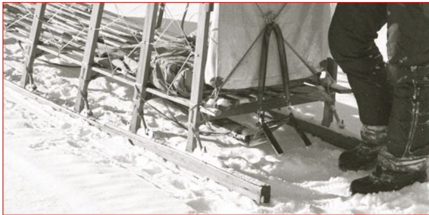
Sasha Wik stands behind her sled. Notice the brake board, side-to-side tether ropes, hinged two-prong brake, and spring. Image: Ole Wik
