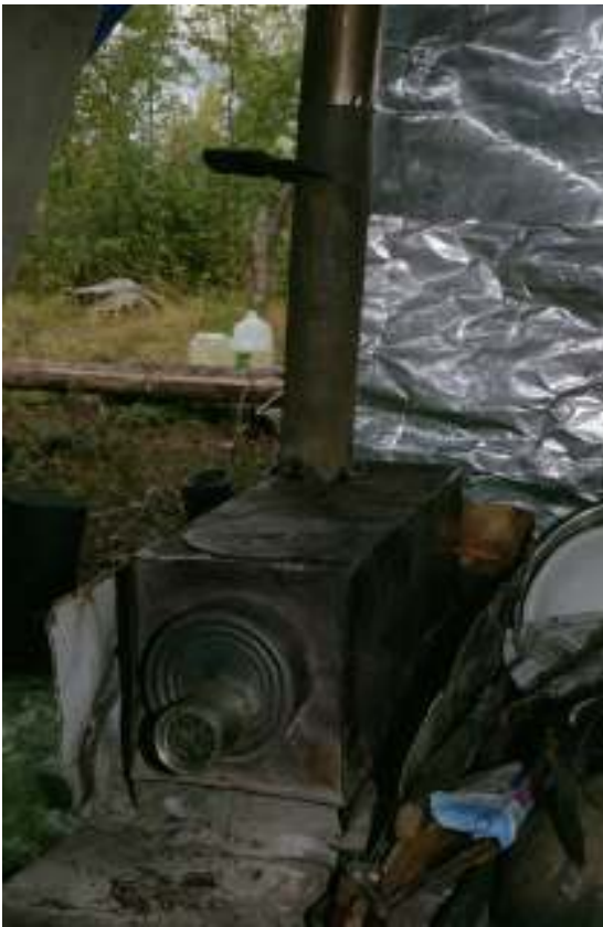
A series of cans makes up the wood stove.
