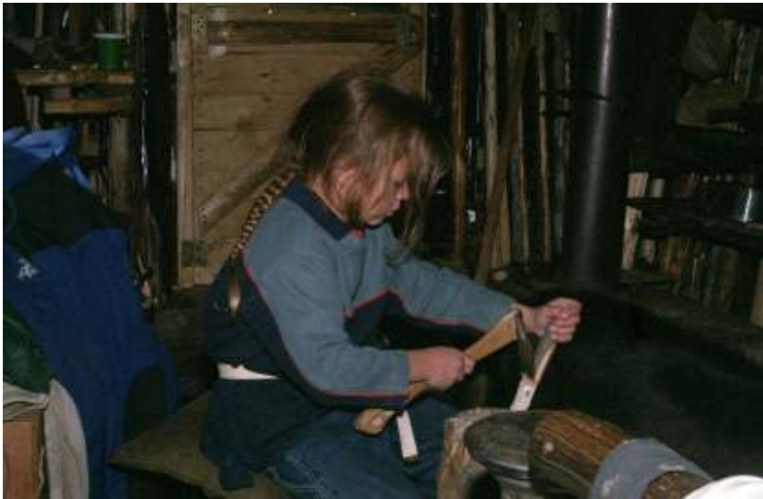
Sharing Oliver's tools is a precious privilege. Sat Sarbat is using a hand adze which Oliver blacksmithed. Notice the holes in the end of the handle to reduce its weight and the graceful curve of the handle making it ergonomically comfortable to use.
